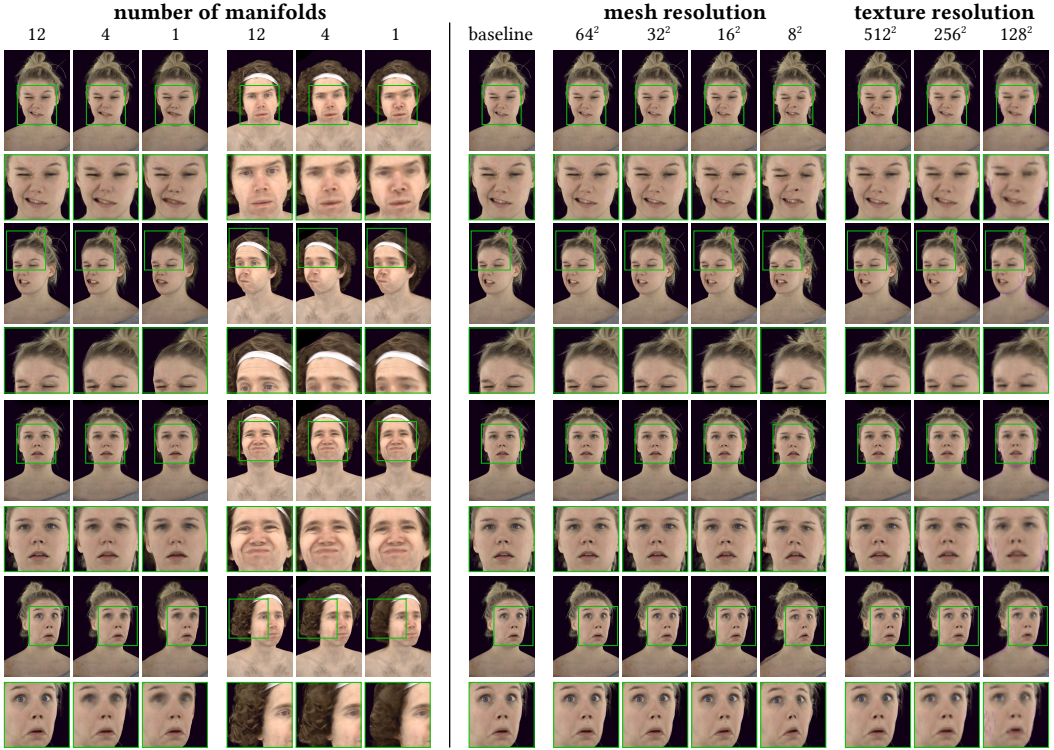
Fig. 7. Ablation results. Number of manifolds. Using a sufficient number of manifolds is essential to attain photorealism and volumetric effects. Mesh resolution. We can decimate the exported meshes to much lower resolutions without sacrificing significant visual quality. Texture resolution. We can modify texture resolution arbitrarily at inference time to trade off image quality with rendering efficiency as desired.
