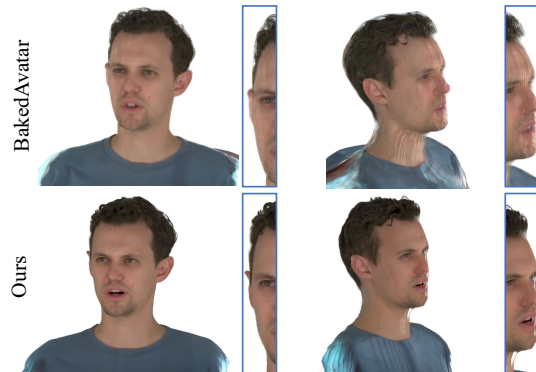
Figure 14. Limitations. Layered mesh representations may suffer from shell artifacts at extreme angles. While our approach outperforms existing baselines on visual quality on novel views at moderate poses ( left ), at more extreme out-of-training profile views ( right ) it also suffers from shell artifacts similar to the baseline.
